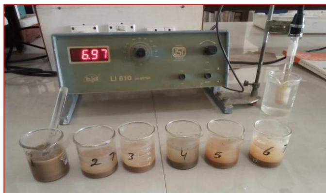
Fig. 3. Measurement of electrical conductivity of soil samples
