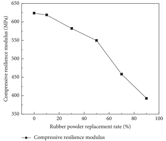
FIGURE 3: Relationship between rubber powder replacement rate and compressive resilience modulus of mixture.
