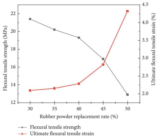
FIGURE 6: Relationship between rubber powder replacement rate and flexural tensile strength of concrete.
