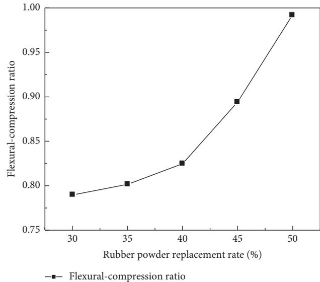
FIGURE 7: Relationship between rubber powder replacement rate and flexural-compression ratio of concrete.
