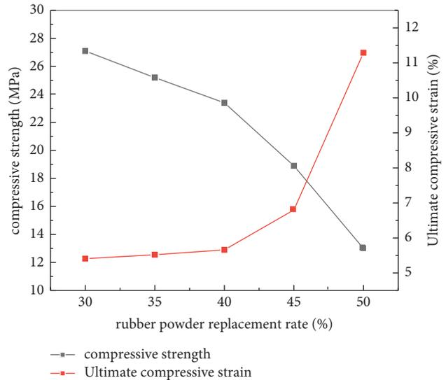
FIGURE 5: Relationship between rubber powder replacement rate and compressive strength of mixture.
