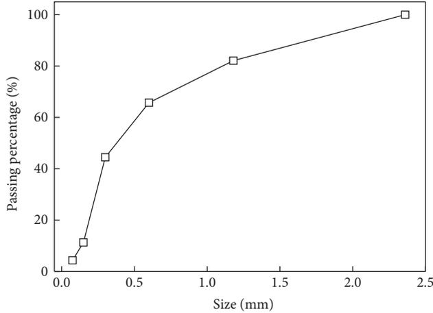
FIGURE 1: Particle size distribution of rubber powder.
