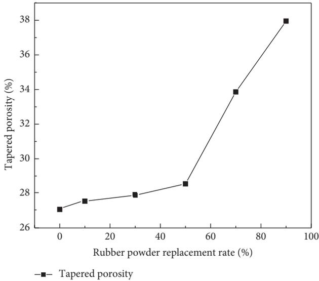
FIGURE 2: Relationship between rubber powder replacement rate and tapped porosity of mixture.
