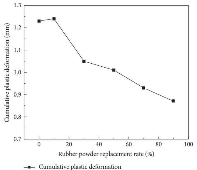
FIGURE 4: Relationship between rubber powder replacement rate and cumulative plastic deformation of mixture.
