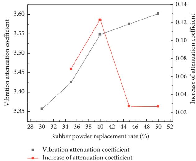
FIGURE 8: Effect of rubber powder replacement rate on vibration characteristics of tire/test piece system.
